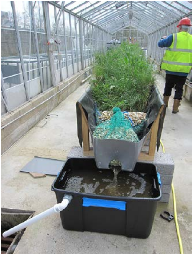
Research undertaken by Portsmouth University, showing water quality improvement by vegetated SuDS components
